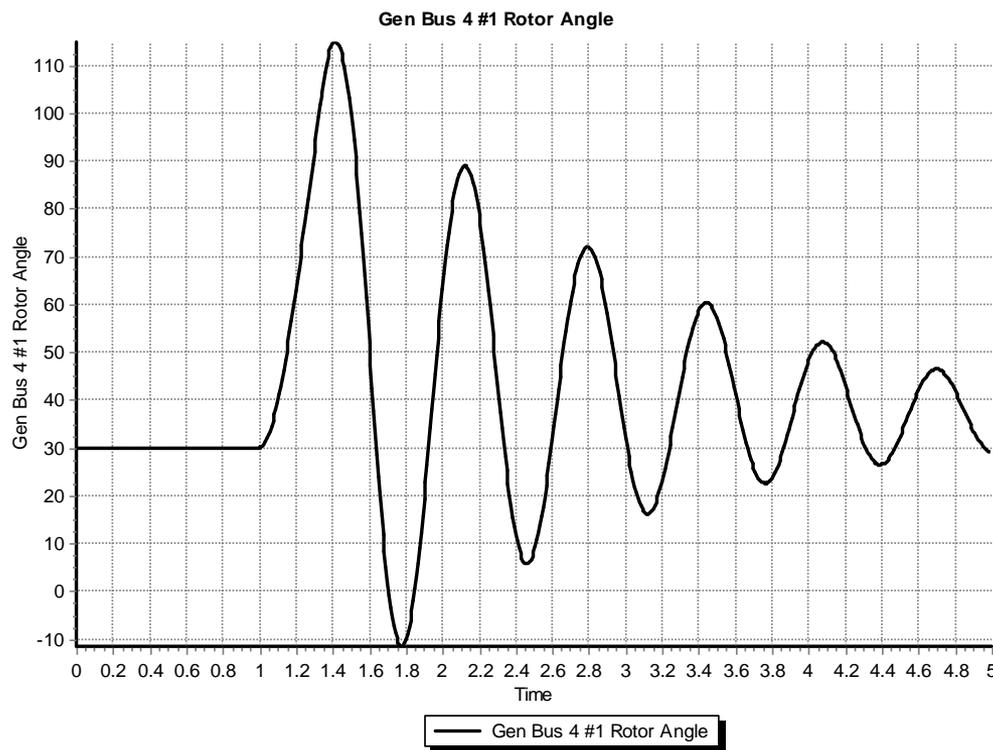
This plot repeats the previous example with the bus 3 fault. The generator response is now damped due to the damper windings included in the GENROU model. Case is saved in examples as **Example\_13\_4\_GENROU**.
