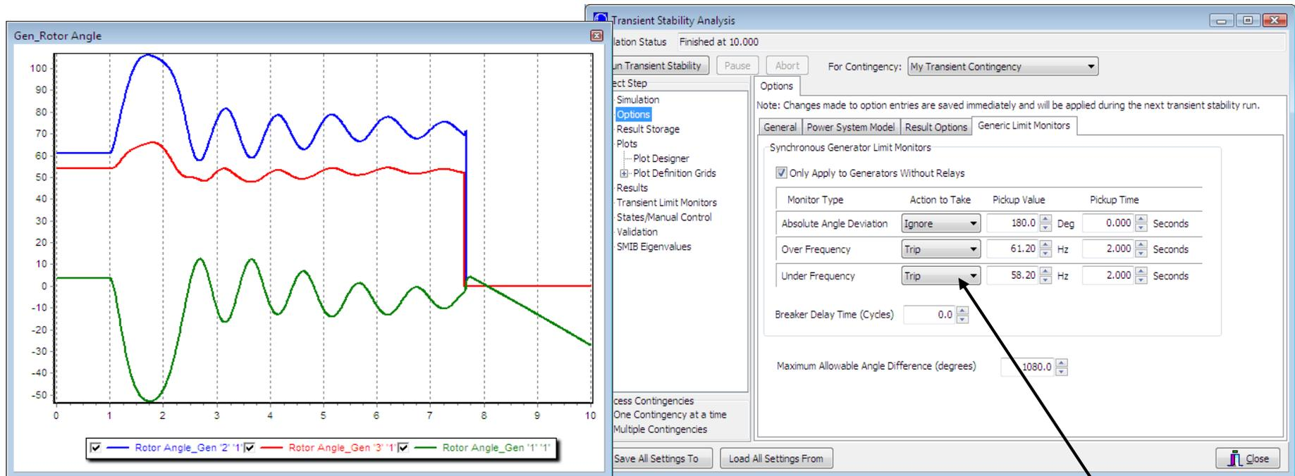
Because this case has no governors and no infinite bus, the bus frequency keeps rising throughout the simulation, even though the rotor angles are stable. Users may set the generators to automatically trip in “Options”, “Generic Limit Monitors”.
