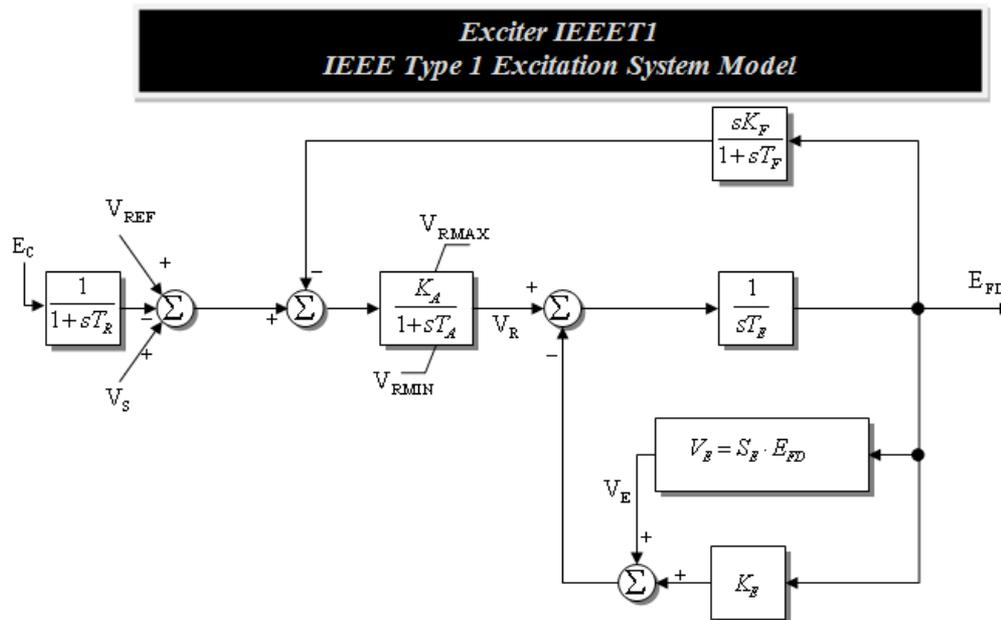
The input to the exciter,  $E_c$ , is usually the terminal voltage. The output,  $E_{FD}$ , is the machine field voltage.
