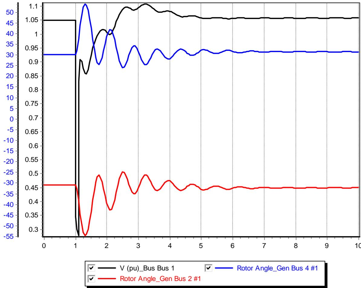
Plot shows the rotor angles for the generators at buses 2 and 4, along with the voltage at bus 1. Notice the two generators are swinging against each other.
