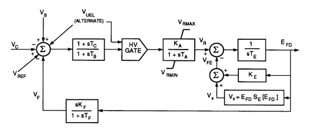
Figure 3—Type DC1A — DC Commutator Exciter
