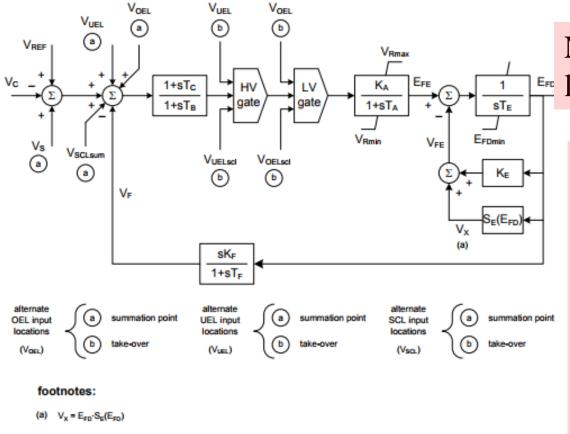
Figure 4—Type DC1C dc commutator exciter
