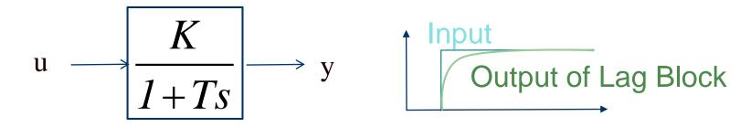
Equation with u as an input and y as an output is
