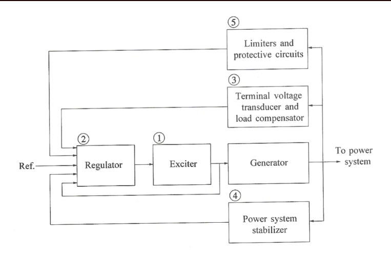
Image source: Fig 8.1 of Kundur, Power System Stability and Control
