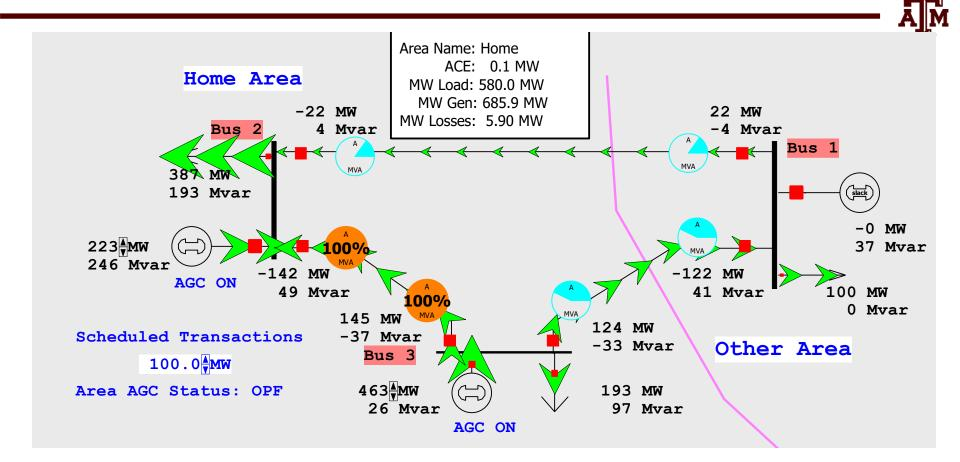
Dispatch is no longer optimal due to need to keep the line from bus 2 to bus 3 from overloading
