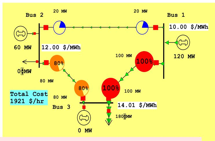
Line from 1 to 3 is no longer overloaded, but now the marginal cost of electricity at bus 3 is \$14 / MWh
