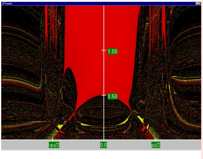
The high solution ROC is actually larger than with the standard NPF. Obviously this is not a good a way to get the low solution
