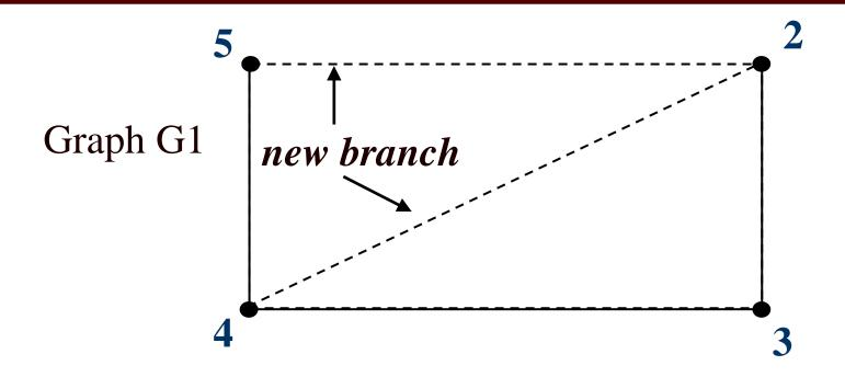
• We obtain the graph G1 from G by removing Bus 1 with the new added branches (2, 4) and (2, 5) corresponding to the fills
