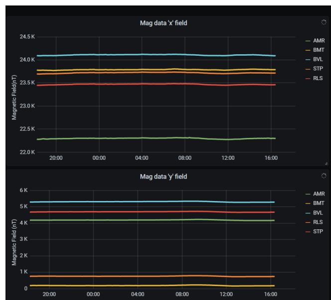
Fig. 10. Real-time magnetometer data looking back over a 20-hr period from June 10th, 4:00 PM on a normal day at multiple stations
