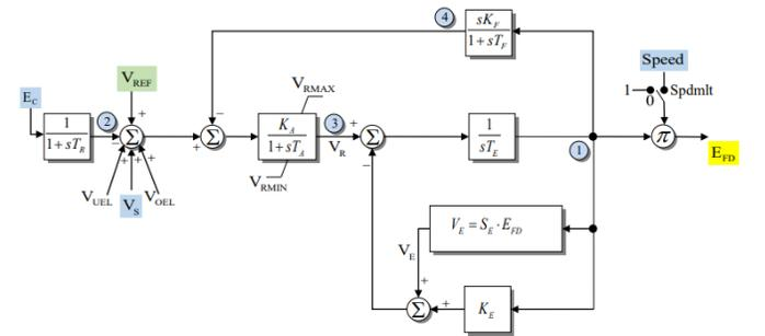
Fig. 4. IEEE1 Exciter Block Diagram [17]
