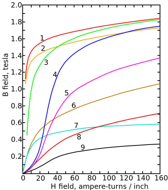
Magnetization curves of 9 ferromagnetic materials, showing saturation. 1. Sheet steel, 2. Silicon steel, 3. Cast steel, 4. Tungsten steel, 5. Magnet steel, 6. Cast iron, 7. Nickel, 8. Cobalt, 9. Magnetite; highest saturation materials can get to around 2.2 or 2.3T
