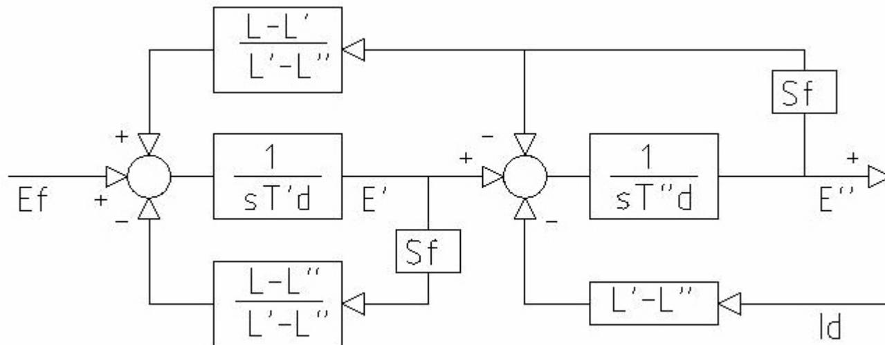
$$S_e = 1 + f_{\text{sat}}(\psi_{\text{ag}} + K_{\text{is}} \cdot I_t)$$
