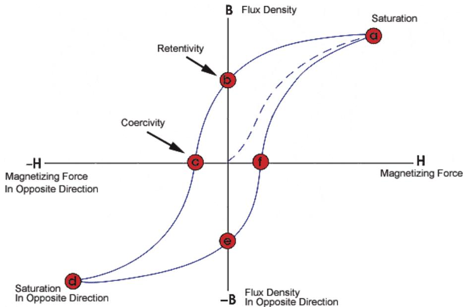
To minimize the amount of magnetic material, and hence cost and weight, electric machines are designed to operate close to saturation
