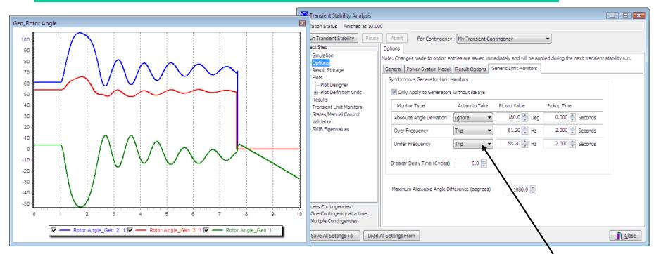
Because this case has no governors and no infinite bus, the bus frequency keeps rising throughout the simulation, even though the rotor angles are stable. Users may set the generators to automatically trip in "Options", "Generic Limit Monitors".
