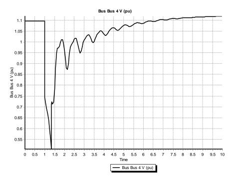
Notice following the fault the voltage does not recover to its pre-fault value. This is because we have not yet modeled an exciter.
