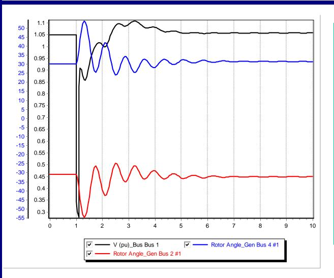
Plot shows the rotor angles for the generators at buses 2 and 4, along with the voltage at bus 1. Notice the two generators are swinging against each other.
