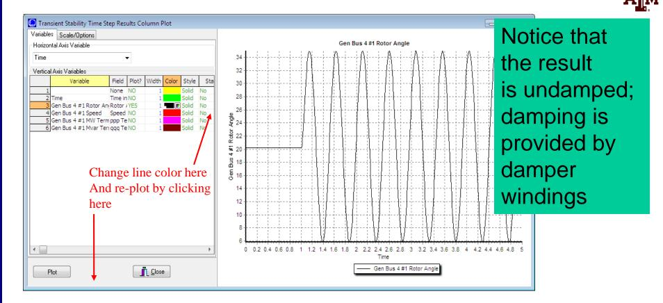
Starting the event at t = 1.0 seconds allows for verification of an initially stable operating point. The small angle oscillation indicates the system is stable, although undamped.
