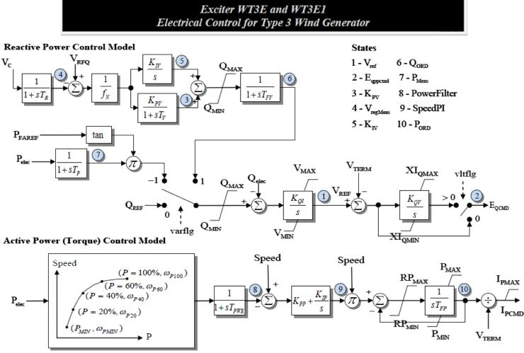
WT3E supported by PSLF with  $RP_{MAX} = P_{wrat}$  and  $RP_{MIN} = -P_{wrat}$ ,  $T_{FV} = T_{C}$
