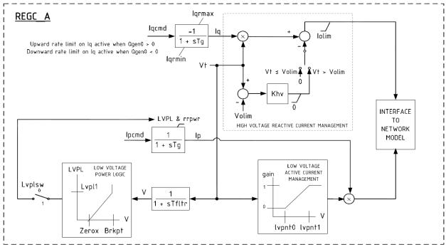
Figure 2. REGC\_A Model Block Diagram
