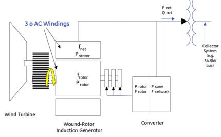
Figure 2-1. GE Doubly Fed Asynchronous WTG Major Components.
