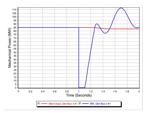
Graph at left shows a zoomed (2 second) view of the gen 3 real power output, with the value falling to zero during the fault, and then ramping back up
