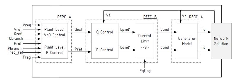
Figure 1. Overall Model Structure for Central Station PV System
