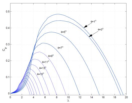
If such a detailed curve is used, the initialization is from the power flow P. There are potentially three independent variables,  $v_w$ ,  $\theta$  and  $\omega$ . One approach is to fix  $\omega$  at rated (e.g., 1.2) and  $\theta$  at  $\theta_{min}$
