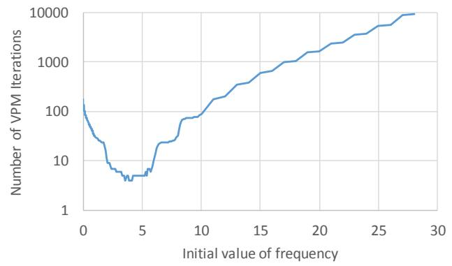
Fig. 7. Sensitivity of case 1 convergence iterations to initial guess of frequency, with the initial guess of damping set to 0.
