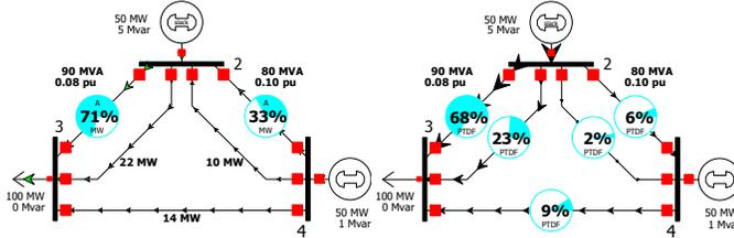
Fig. 2. Reduced 3-bus case with line loading (left) and PTDFs from bus 2 to bus 3 (right)
