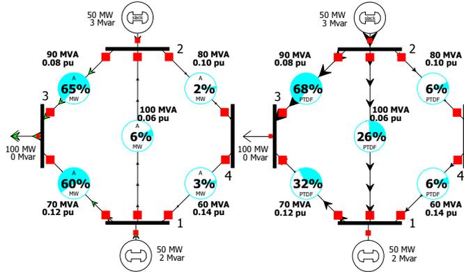
Fig. 3. Full 4-bus case with line loading (left) and PTDf values from bus 2 to bus 3 (right)
