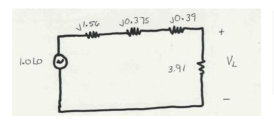
Convert to per unit as before. Note the system is exactly the same!
