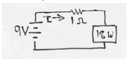
where the 18 watt load is a resistive load
