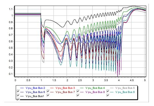
The models are no longer giving realistic results; two generators trip on over speed; then the load trips after 4 seconds.
