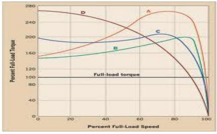
Class B machines should have a lower starting current compared to A (500% rated versus 800% for B) In steady-state the motor will operate on the right side of the curve at the point at which the electrical torque matches the mechanical torque
