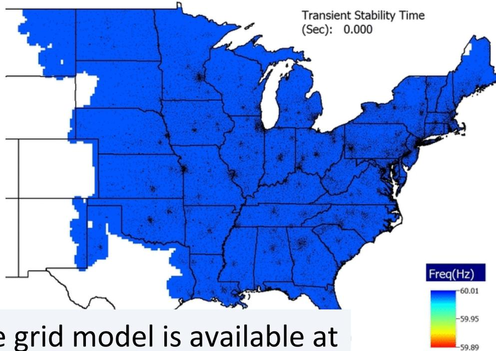
These results were created using a 70K bus system with detailed dynamic models for 8000 generators. The models and all the data associated with this image are public
