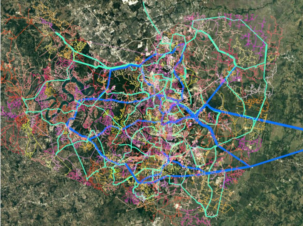
This is a synthetic grid, but utilizing a quite realistic layout; blue is 230 kV, light green 69 kV, and lots of distribution lines down to hundreds of thousands of electric meters.
