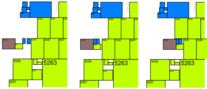
Fig. 6. The effect of the choice of pushing distance. The brown tile is being pushed from left to right. Left, before pushing. Center, smaller pushing distance. Right, larger pushing distance.
