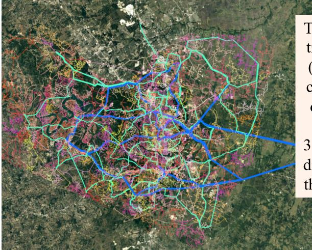
The figure shows the transmission system (blue is 230 kV and cyan 69 kV) and the distribution system modeled down to 307,000 meters. The distribution data is in the OpenDSS format.
