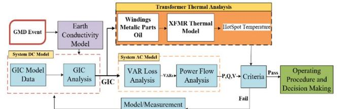
Fig. 1. Overall architecture suggested for thermal analysis of power grid transformers impacted by GICs.
