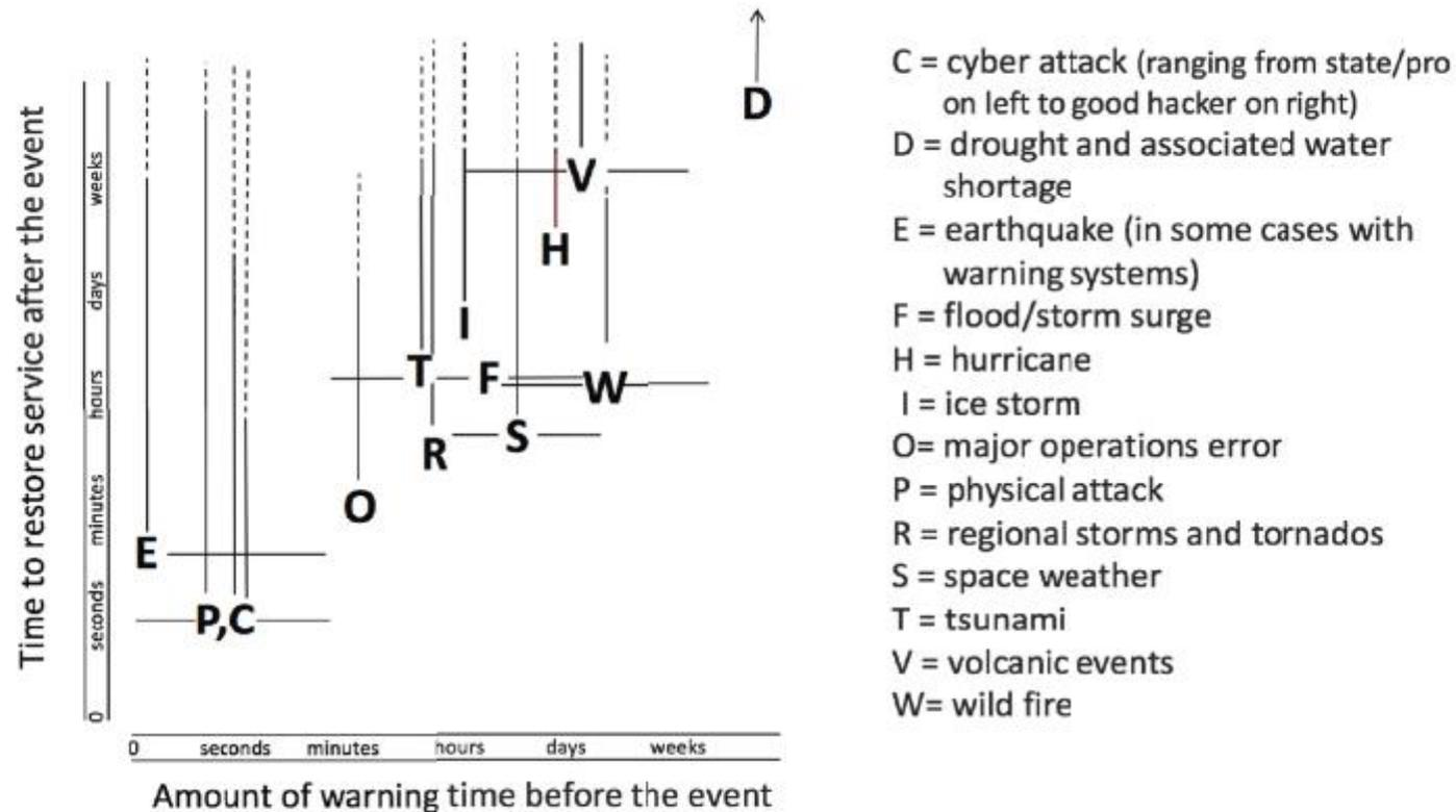
**FIGURE 3.1** Mapping of events that can cause disruption of power systems. The horizontal placement provides some indication of how much warning time there may be before the event. The vertical axis provides some indication of how long it may take to recover after the event. Lines provide a representation
