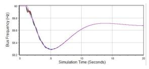
Figure 2: Example 37-Bus Frequency Response
