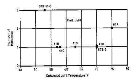
Graph used to determine whether to launch Challenger in 1986; shows O-ring failure vs. temperature but neglects launches with no failures
