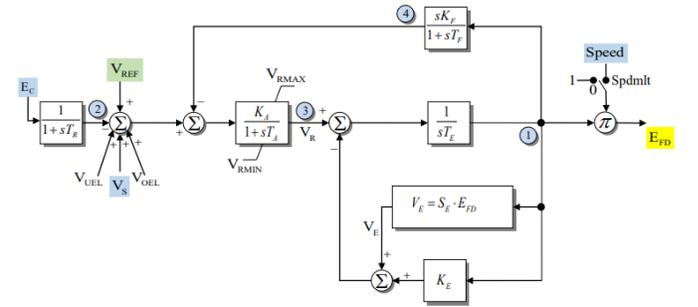
Fig. 4. IEEE1 Exciter Block Diagram [17]
