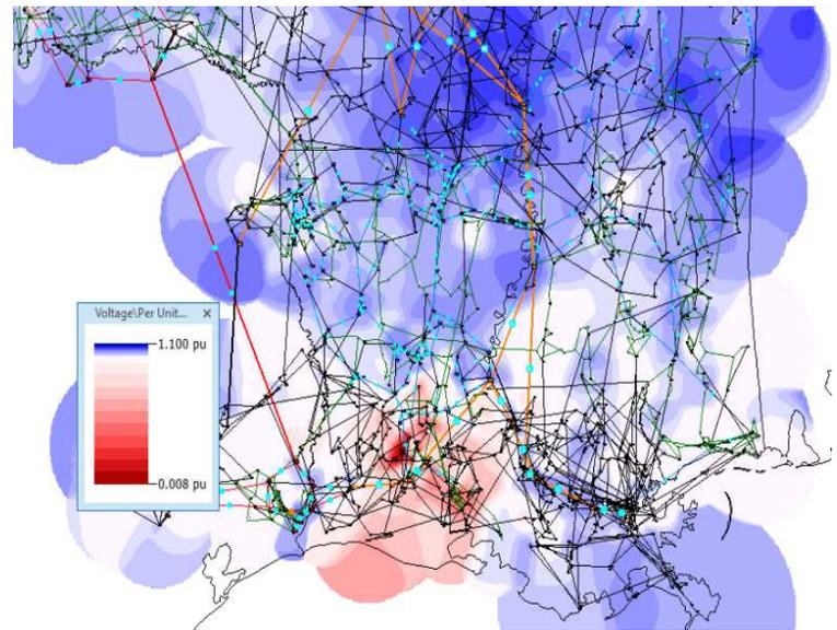
Fig. 9. Showing a low-voltage solution of 27k-bus system.
