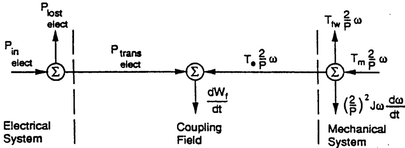
The coupling field stores and discharges energy but has no losses
