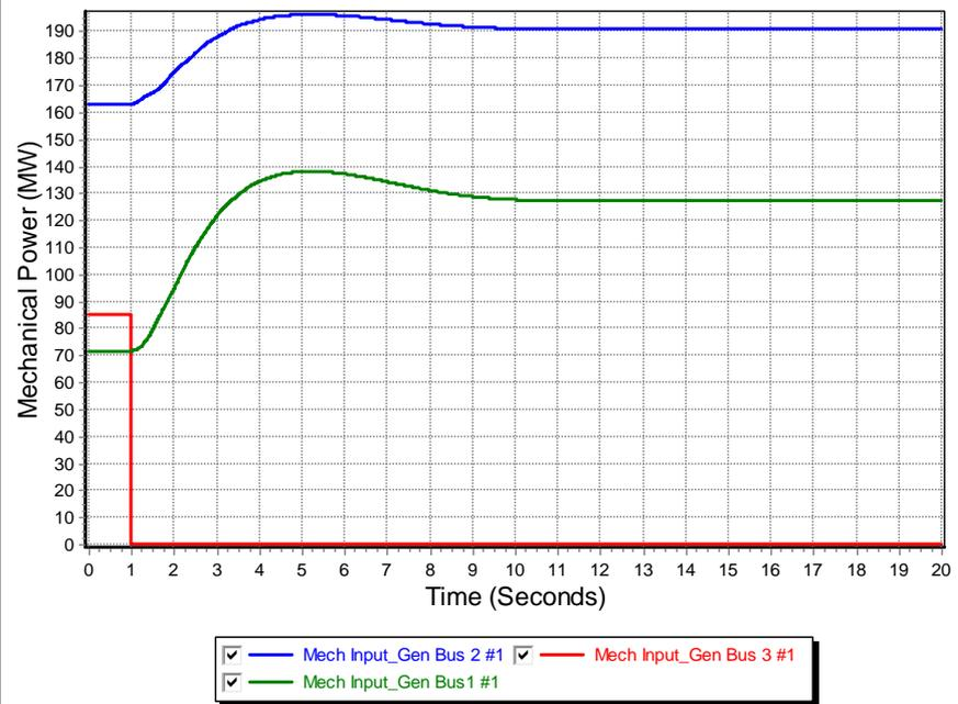
The left figure shows the generator speed, while the right figure shows the generator mechanical power inputs for the loss of generator 3. This is a severe contingency since more than 25% of the system generation is lost, resulting in a frequency dip of almost one Hz. Notice frequency does not return to 60 Hz.
