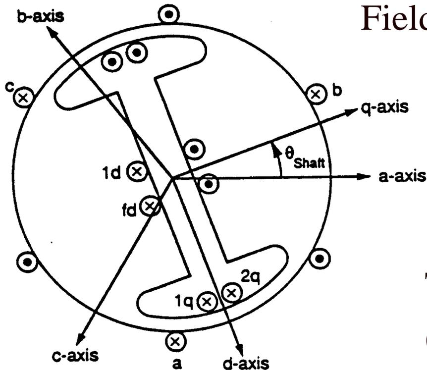
Field winding (fd) on rotor
