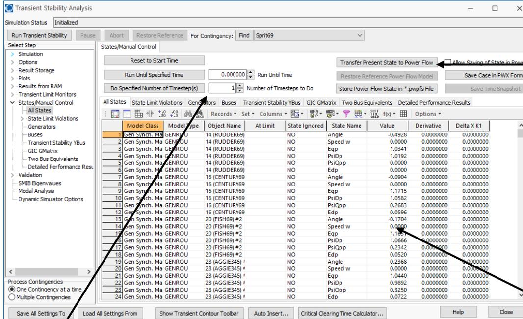
Transfer results to Power Flow to view using standard PowerWorld displays and one-lines
