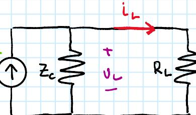
$$I_s = i_L (t - d/v_p) - \frac{1}{Z_c} v_k (t - d/v_p)$$
