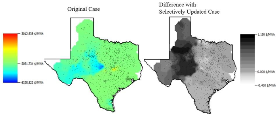
Fig. 5: Bus LMPs in OPF solution for original 2,000 bus base case (left). Difference contours with comparison to base for selectively updated case (right).
