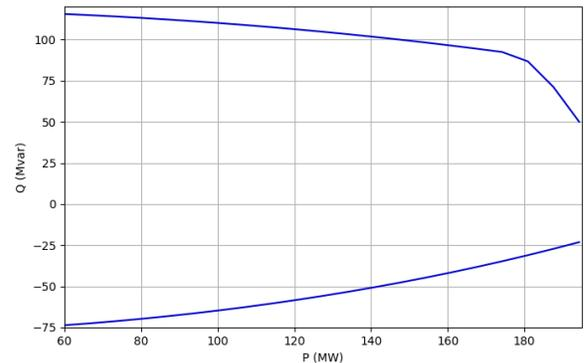
Fig. 4: An example of generator capability curve: Bus 1053 in 2000 bus case.
