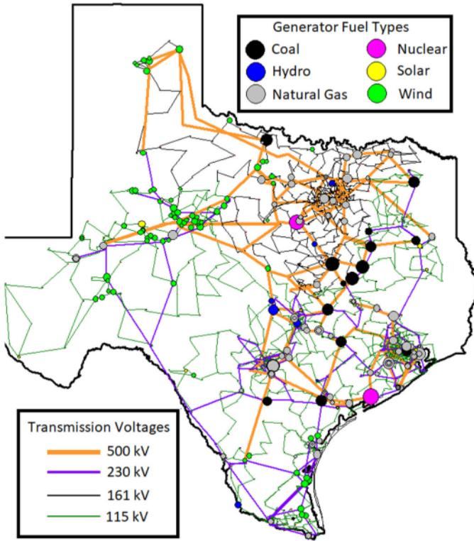
Fig. 1. Synthetic 2000-bus test case oneline diagram [3], [4]. Transmission voltages are shown, as well as circles representing the generators, with color indicating fuel type and size indicating the relative MW capacity. This grid is fictitious and does not represent the actual Texas grid.
