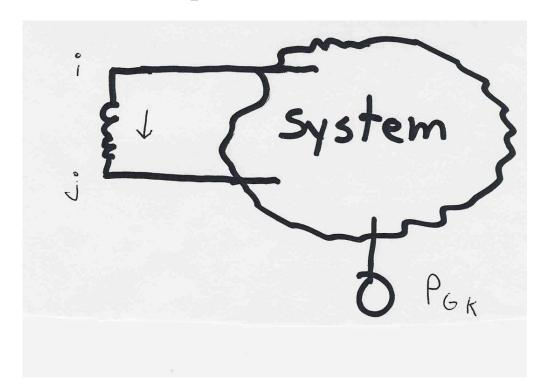
The assumption is that the change in generation is absorbed by the slack bus
