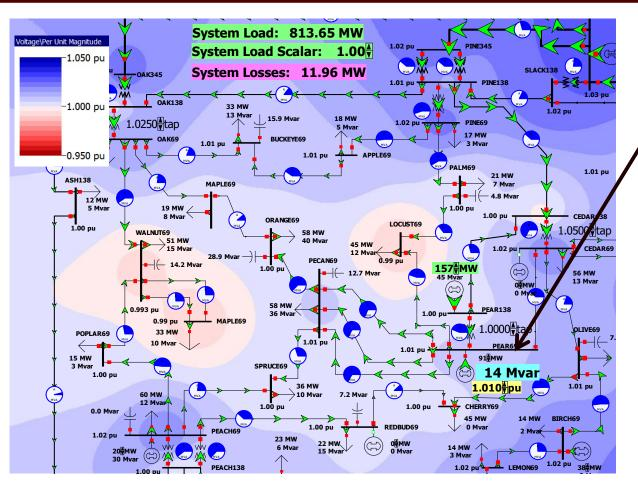
This example uses the case **PSC\_37Bus** with a voltage contour. Try varying the voltage setpoint for the generator at PEAR69
