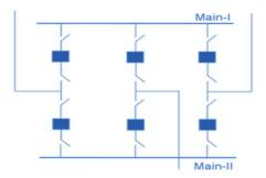
Fig D: Double Bus Double Breaker
