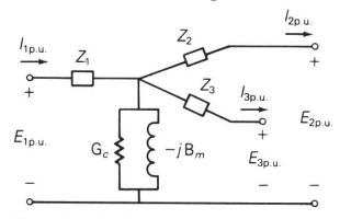
Per-unit equivalent circuit—practical transformer
