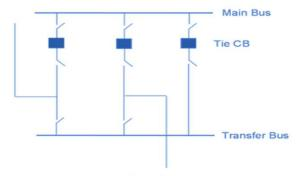
Fig C: Main and Transfer Bus
