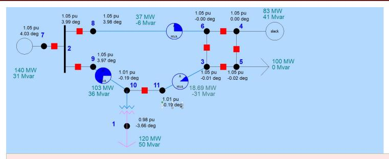
Case name is **FT\_11Node**. PowerWorld consolidates nodes (buses) into super buses; available in the Model Explorer: Solution, Details, Superbuses.
