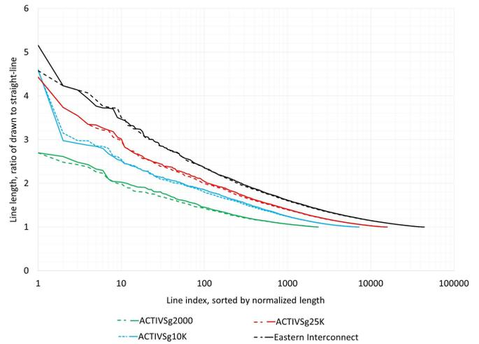
Fig. 12. Distribution of transmission line drawn length, relative to a straight-line distance. The lines are plotted in sorted order. Dashed lines and solid lines show the Delaunay algorithm one- and two-level for the four cases.
