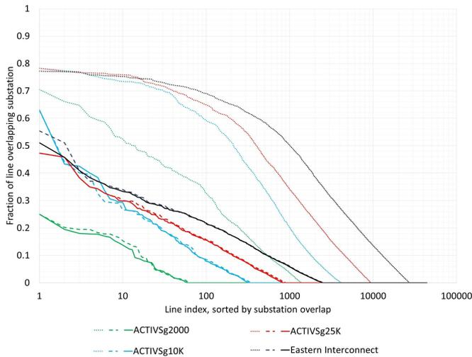
Fig. 11. Distribution of transmission line overlap. The lines are plotted by fraction of overlap with substations, in sorted order. Dotted lines show the original overlap, dashed lines and solid lines show the Delaunay algorithm one-level and two-level.
