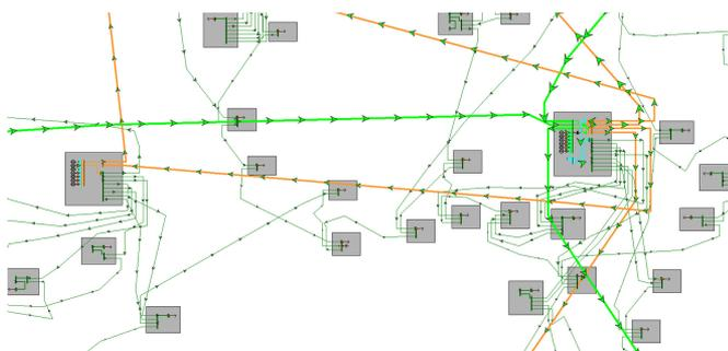
Fig. 7. A Two-layer Delaunay approach to drawing transmission lines, which avoids both overlapping substations and excessive bends in the high-voltage lines.
