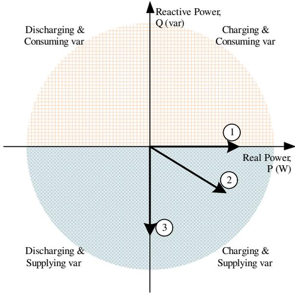
Figure 5: Modes of operation (load notation:  $P_L + jQ_L$ )
