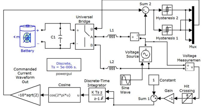
Figure 6. Simulink block diagram of the battery-inverter device
