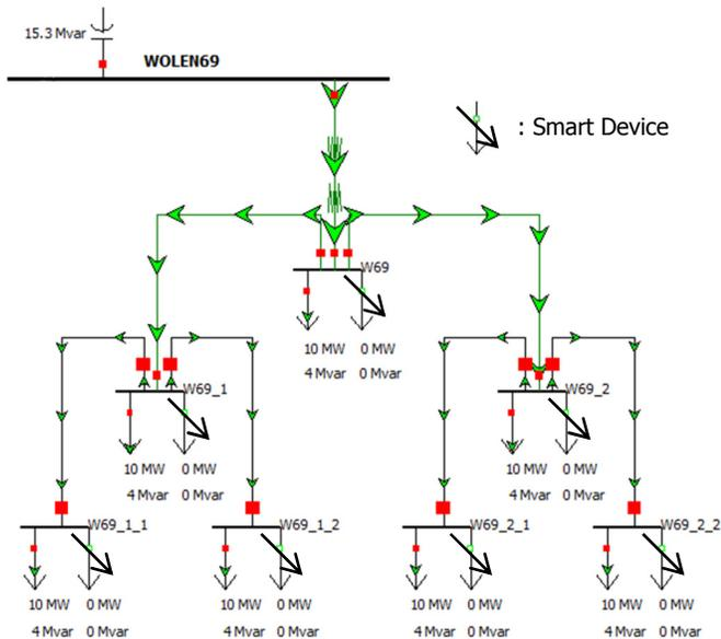
Figure 4. 13.8kV Sub-network of WOLEN69
