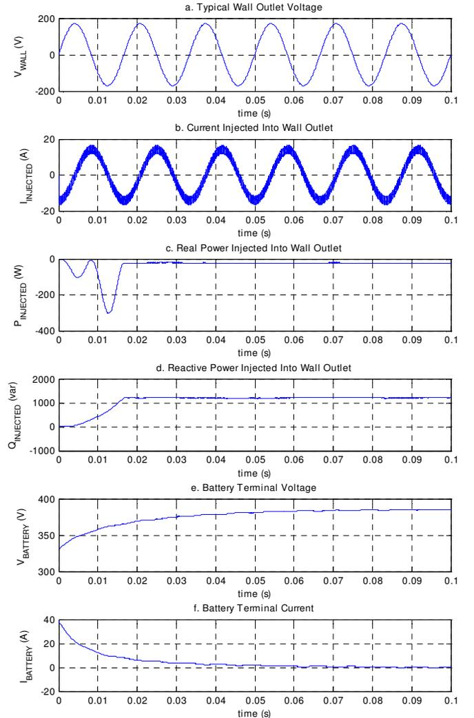
Figure 7: Battery-inverter device simulation results (injected notation)
