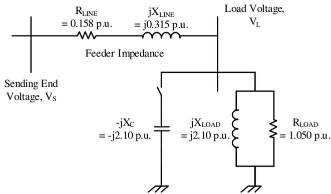
Figure 2. Shunt capacitor (switched out) at the end of a primary feeder ( $S_{base\phi} = 10 \text{ MVA}$  &  $V_{baseLL} = 13.8 \text{ kV}$ )
