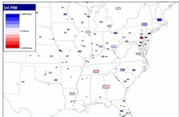
Figure 4: Figure 3 Display with Rectangle Color Based on Area Interchange (Exports are Blue, Imports are Red)
