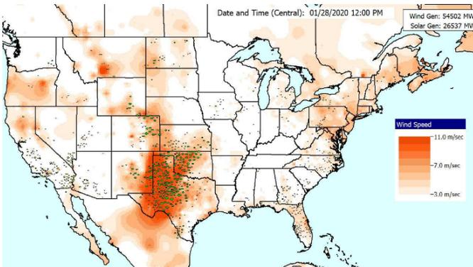
Fig. 5: Wind Speed Contour and Wind Generator Power Outputs
