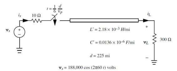
for  $0 \le t \le 0.04$  sec using a time step of  $\Delta t = \frac{1}{6} \frac{d}{\nu_p}$ . Plot  $v_L$ .
