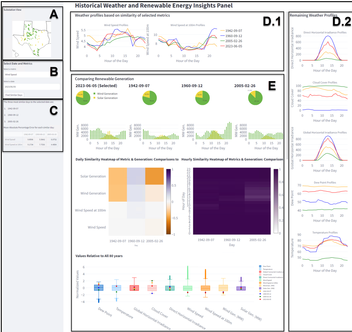
Figure 1: Screenshot showing the Historical Weather & Renewable Energy Insights panel where the five sections are alphabetically labeled. A: Static image of the substation layout on the geographic footprint of Texas; B: User-selectable inputs (date, metrics by which to find similar days); C: Outputs with the three most similar days to the selected date; D.1: Weather profiles for user-selected metrics by which similarity is calculated; D.2: Rest of the weather profiles for the four days; E: Wind and Solar generation output.
